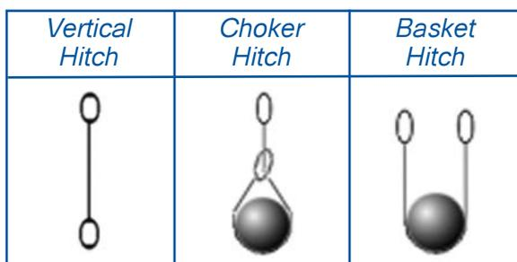
Push both forks of the forklift as close together as possible in the center of the forklift. Position forklift forks above the ramp. Feed the sling through the side mounted lifting lug and position one loop of the sling over each fork to within 24 inches of the forklift carriage, thus creating a basket lift. Lift the yard ramp until it clears the floor of the trailer by a few inches. Move away from the trailer and lower the ramp to the ground.
