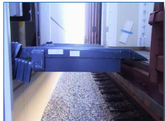
RAILBOARD IN USE
