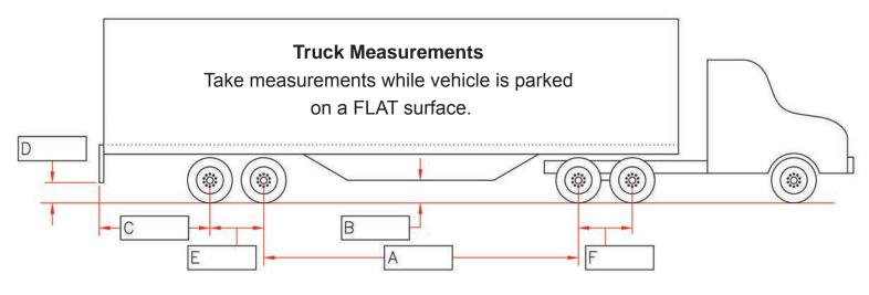
Dimension A: axle to axle span
