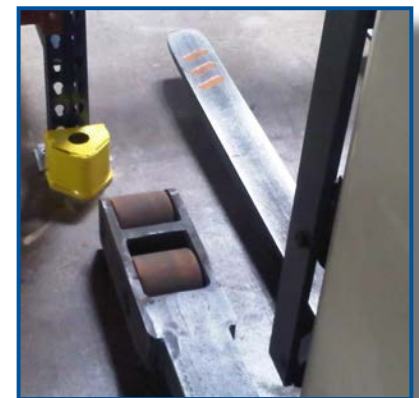
The rack above is protected by the Bullnose Guard.
